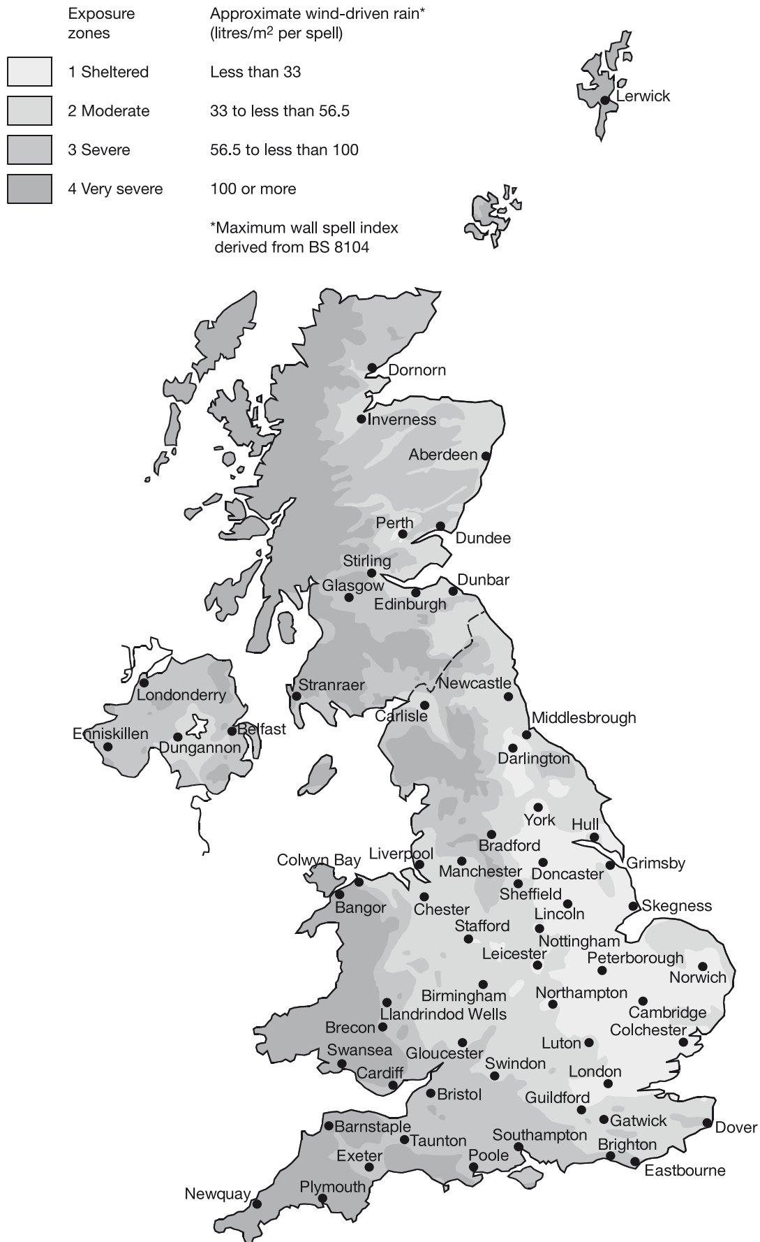
Diagram 12 UK zones for exposure to driving rain
